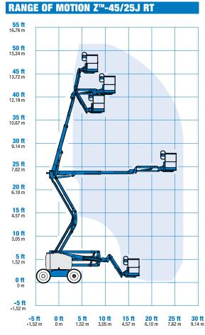
$<sup>^{\</sup>star}$ The metric equivalent of working height adds 2 m to platform height. U.S. adds 6 ft to platform height.
